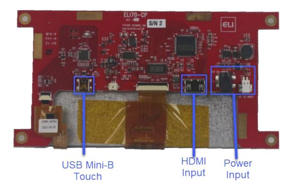
Power may be supplied either via the 2-pin terminal block J4 or via the 2.1mm power jack P2 (center positive)
