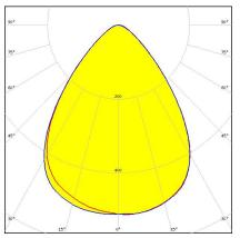
Dimensions: 53.9 mm x 53.9 mm Height: 17.00 mm ~90° wide beam with holder C compatible with LEDiL HEKLA
