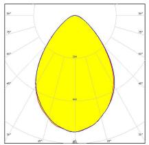
Dimensions: 69.9 mm x 69.9 mm Height: 14.60 mm ~90° very wide beam with holder B compatible with 3rd party connectors from BJB, IDEAL and Stucchi.
