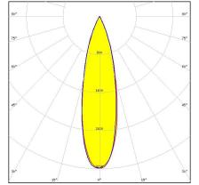
Dimensions: 69.9 mm x 69.9 mm Height: 14.60 mm ~25° spot beam with holder B compatible with 3rd party connectors from BJB, IDEAL and Stucchi
