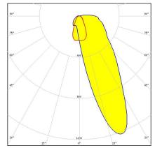
Dimensions: 53.9 mm x 53.9 mm Height: 24.65 mm Asymmetric beam for wall washing with holder C compatible with LEDiL HEKLA
