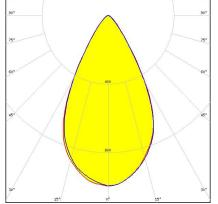
Dimensions: 53.9 mm x 53.9 mm Height: 16.90 mm ~60° wide beam with holder C compatible with LEDiL HEKLA
