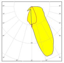
Dimensions: 69.9 mm x 69.9 mm Height: 21.80 mm Asymmetric beam for wall washing
