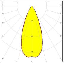
Dimensions: 52.1 mm x 52.1 mm Height: 16.98 mm ~45° wide beam with holder C compatible with LEDiL HEKLA
