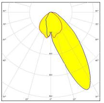
Dimensions: 53.9 mm x 53.9 mm Height: 16.00 mm Asymmetric beam ideal for floor installations with holder C compatible with LEDiL HEKLA
