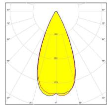
**Dimensions: 69.9 mm x 69.9 mm Height: 14.00 mm** ~45° wide beam with holder A
