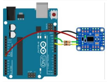
Connect V+ to 4-17V and keep VCC disconnected. Then use 10K resistors or a level shifter between the clock and data wires going into the *first* of the TLC59711
