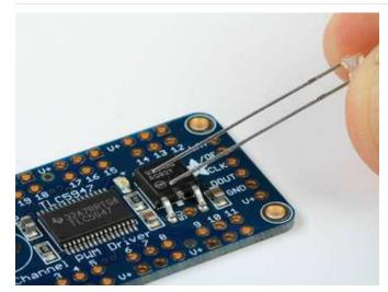
Connecting Monochrome LEDs Note that one leg of the led is longer than the other. This is the Anode and should be connected to the V+hole in the board.
