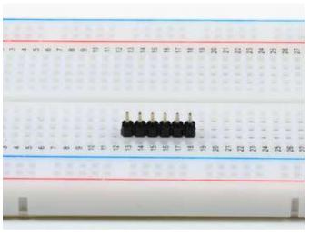
Position the header Cut to size first if necessary
