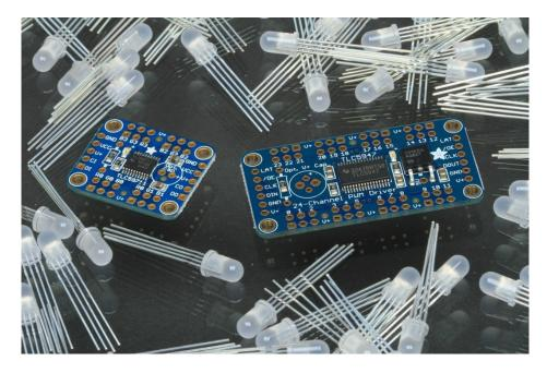
The **TLC59711** can control 12 separate channels of 16-bit PWM output. This is the highest-resolution PWM board we've seen!
