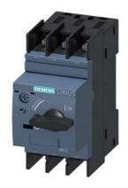
Circuit breaker size S00 for motor protection, CLASS 10 A-release 0.28...0.4 A N-release 5.2 A ring cable lug connection Standard switching capacity
