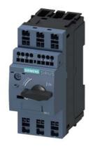
Circuit breaker size S00 for motor protection, CLASS 10 A-release 0.55...0.8 A N-release 10 A Spring-type terminal Standard switching capacity with transverse auxiliary switches 1 NO+1 NC
