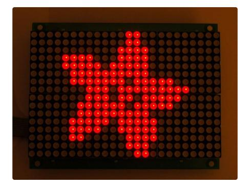
These LED panels take care of all the work of making a big matrix display. Each panel has six 8x8 red matrix modules, for a 16x24 matrix. The panel has a HT1632C chip on the back with does all the multiplexing work for you and has a 3-pin SPI-like serial interface to talk to it and set LEDs on or off. There's a few extras as well, such as being able to change the brightness of the entire display, or blink the entire display at 1 Hz.
