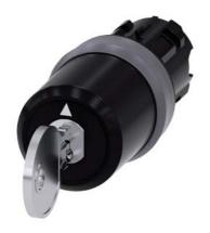
Key-operated switch BKS, 22 mm, round, plastic with metal front ring, lock number S1, with 2 keys, 3 switch positions I>O<II, momentary contact on the left, latching on the right, actuating angle 2x45°, 10:30h/12h/13:30h, key removal O, with laser labeling, lower case
