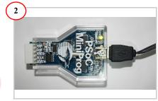
Remove the CY3217-MiniProg1 from the kit package; plug the USB cable into the USB Mini B connector and connect it to your PC.
