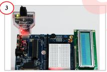
Connect the MiniProg1 to the ISSP header on your target PSoC board.
