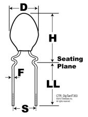
**General Information** Series T353 Dielectric MnO2 Tantalum Style Radial Description Radial, Solid Tantalum, Conformal, Dipped Features Low Leakage RoHS No MARNING: Cancer and reproductive harm -Prop 65 http://www.p65warnings.ca.gov. SCIP 0c1392c3-c7b9-4178-827c-fa26617a3178 Number Termination Lead (SnPb) AEC-Q200 No Notes Longest Lead Is Positive.
