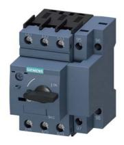
Circuit breaker size S0 for motor protection, CLASS 10 with overload relay function A-release 13...20 A N-release 260 A screw terminal Standard switching capacity
