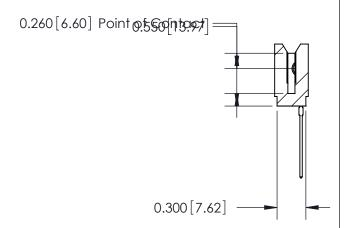
745 Series Ultra-Mate Card Edge Connector - Press Fit Part Number: 745-051-541-106
