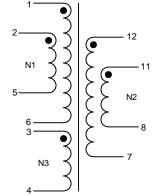
N1, N2 denotes two windings connected in parallel. Terminals 1+2, 5+6, 7+8 and 11+12 must be tied as solder bridging is allowed.
