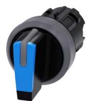
Selector switch, illuminable, 22 mm, round, plastic with metal front ring, blue, selector switch, short, 3 switch positions I>O<II, momentary contact type, actuating angle  $2x45^{\circ}$ , 10:30h/12h/13:30h, with laser labeling, upper case and lower case, always upper case at beginning of line
