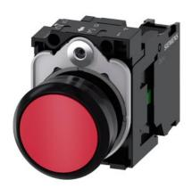
Pushbutton, 22 mm, round, plastic, red, pushbutton, flat, momentary contact type, with holder 1 NO, screw terminal, with laser labeling, symbol number according to, ISO 7000 or IEC 60417
