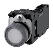
Illuminated pushbutton, 22 mm, round, plastic with metal front ring, clear, pushbutton, flat, momentary contact type, with holder, 1 NO+1 NC, LED module with integrated LED 24 V AC/DC, screw terminal, with laser labeling, inscription or symbol Customer-specific selection with SIRIUS ACT configurator (CIN)
