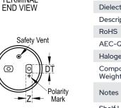
**General Information** Series **PEH200** Dielectric Aluminum Electrolytic Description Screw Terminal, Aluminum Electrolytic Yes AEC-Q200 No Halogen Free Yes Component 415 g Weight Dimensions D And L Include Sleeving. MS (MxS) = M12x16. Shelf Life 156 Weeks
