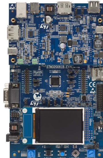
Figure 2. STM32G081B-EVAL board with UCPD daughterboard
