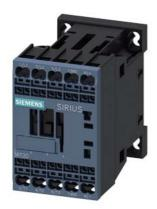
power contactor, AC-3 9 A, 4 kW / 400 V 1 NO, 24 V DC 0.7-1.25\*Us 3-pole, size S00 spring-type terminal with integrated suppressor diode spring-type terminal suitable for PLC outputs not expandable with auxiliary switch
