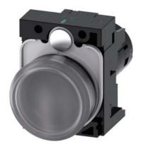
Indicator light with LED lamp, compact, 22 mm, round, plastic, clear with red-yellow-green LED, lens, smooth, with holder, operating voltage 6-24 V AC/DC, screw terminal, with laser labeling, lower case
