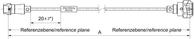
All dimensions are in mm; tolerances:  $\pm$  3mm for A  $\leq$  300 mm;  $\pm$  1% for A > 300 mm \*) If length "A"  $\leq$  90 mm marking is mount centric  $\pm$  5mm
