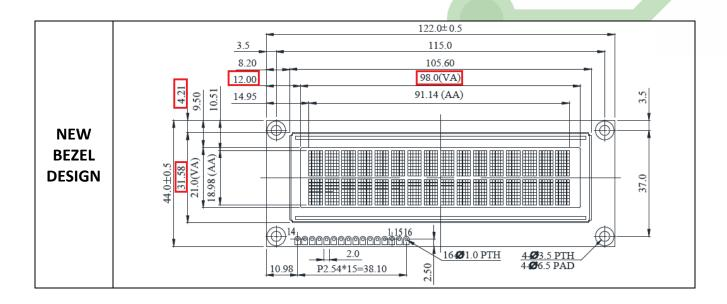
Overall Bezel Height has been reduced from 34.2mm to 31.58mm. Horizontal Viewing Area has been reduced from 99.0mm to 98.0mm. Active Area (visible character area) has remained unchanged.
