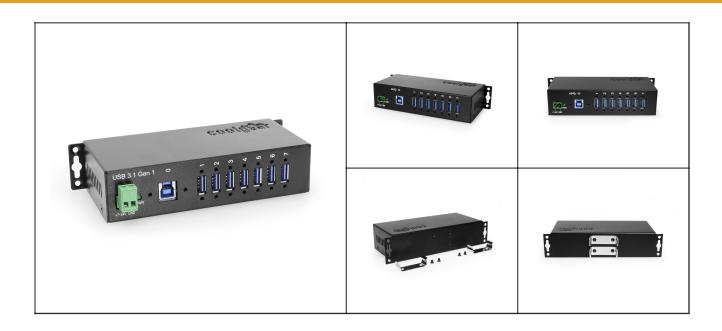
USB 3 7-Port hub with built-in single chip USB3.0 controller and provides an unique feature to work in the bus-powered mode without an external AC power adapter. The external DC jack is used for self-powered mode if you need more power on the 7 downstream ports.
