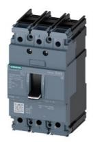
circuit breaker 3VA5 UL frame 125 breaking capacity class S 25kA @ 480 V 3-pole, line protection TM210, FTFM, In=100A overload protection Ir=100A fixed short-circuit protection Ii=10 x In UL489 SB (naval), 50 deg. cel. nut keeper kit on both sides
