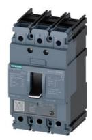
circuit breaker 3VA5 UL frame 125 breaking capacity class M 35kA @ 480 V 3-pole, line protection TM230, FTAM, In=35A overload protection Ir=35A fixed short-circuit protection Ii=5...10 x In nut keeper kit on both sides
