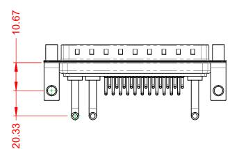
**OPERATING TEMPERATURE:** -55°C ~ 125°C 20A (CURRENT) POWER/CO-AX CONTACT RATING: (IF PRESENT) SIGNAL CONTACT CURRENT RATING: 5A PER CONTACT SIGNAL CONTACT RESISTANCE:  $10m\Omega$  MAX. **INSULATOR RESISTANCE:** 5000MΩ min. DIELECTRIC
