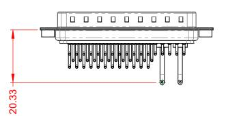
POWER/CO-AX CONTACT RATING:10A (CURRENT)(IF PRESENT)SIGNAL CONTACT CURRENT RATING:5A PER CONTACTSIGNAL CONTACT RESISTANCE:10mΩ MAX.INSULATOR RESISTANCE:5000MΩ min.DIELECTRIC5000MΩ min.
