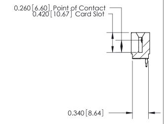
726 Series Ultra-Mate Card Edge Connector - Press Fit
