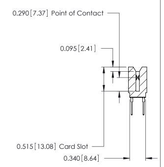
ACAD REFERENCE NO. 746 Series Ultra-Mate Card Edge Connector - Press Fit DRAWN: J.LEE Part Number: 746-042-527-206 CHECKED: **EDAC INC** SCALE: THESE DRAWINGS AND SPECIFICATIONS ARE THE PROPERTY OF EDAC INC.,AND TORONTO, ONTARIO SHALL NOT BE REPRODUCED, OR COPIED DRAWING NUMBER CANADA OR USED AS THE BASIS FOR THE 746-ENG MASTER MANUFACTURE OR SALE OF APPARATUS YOUR CONNECTION TO QUALITY & SERVICE WITHOUT WRITTEN PERMISSION.
