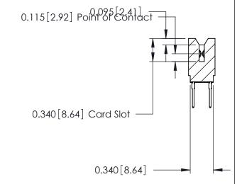
ACAD REFERENCE NO. 746 Series Ultra-Mate Card Edge Connector - Press Fit DRAWN: Part Number: 746-076-527-606 CHECKED: **EDAC INC** THESE DRAWINGS AND SPECIFICATIONS ARE THE PROPERTY OF EDAC INC.,AND TORONTO, ONTARIO SHALL NOT BE REPRODUCED, OR COPIED CANADA OR USED AS THE BASIS FOR THE MANUFACTURE OR SALE OF APPARATUS
