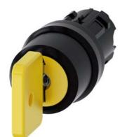
Key-operated switch O.M.R, 22 mm, round, plastic, lock number 73033, yellow, with 2 keys, 3 switch positions I-O-II, latching, actuating angle 2x45°, 10:30h/12h/13:30h, Key removal I+O+II Z=50-unit packaging
