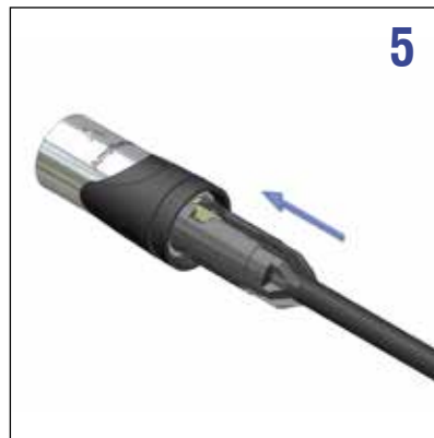
Align the key of the insert with the keyway on the shell then push the pin insert & cable clamp together in the shell.
