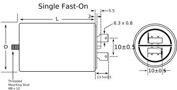
Plastic Case and Cover, Ultra Sonically Welded Description Ultra Sonically Welded Seal, Safety Class PO, Features UL 94 V0 Disk **RoHS** Yes Lead Fast On (1+1) UL, VDE, UL (Construction Only), UL\_94 VO Qualifications Disk AEC-Q200 No Component 38 g Weight
