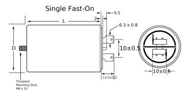
General Information Series C27 Dielectric Film/Foil Polypropylene Style Plastic Case and Cover, Ultra Sonically Welded Description Ultra Sonically Welded Seal, Safety Class PO, Features UL 94 V0 Disk **RoHS** Yes Lead Fast On (1+1) UL, VDE, UL (Construction Only), UL\_94 VO Qualifications Disk AEC-Q200 No Component 68 g Weight
