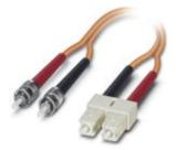
Assembled FO cable, zip cord cable, multi-mode fiberglass 62.5/125 µm, OM1, connector: SC duplex/B-FOC (ST), degree of protection: IP20, for installation in cable ducts or control cabinets
