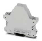
DIN rail housing, Lower housing part with metal foot catch, flat design, with vents, width: 22.5 mm, cross connection: integrated bus connector, number of positions cross connector: 10+2
