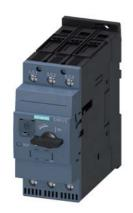
Special type Circuit breaker size S2 for motor protection, CLASS 10 A-release 54...65 A N-release 845 A screw terminal Standard switching capacity Ambient temperature -50  $^{\circ}\text{C}$  250 switching cycles
