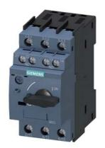
Circuit breaker size S00 for transformer protection A-release 0.11...0.16 A N-release 3.3 A screw terminal Standard switching capacity with transverse auxiliary switches 1 NO+1 NC  $\,$
