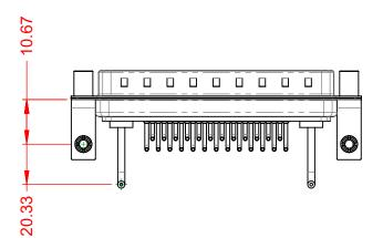
**OPERATING TEMPERATURE:** -55°C ~ 125°C 10A (CURRENT) POWER/CO-AX CONTACT RATING: (IF PRESENT) SIGNAL CONTACT CURRENT RATING: 5A PER CONTACT SIGNAL CONTACT RESISTANCE:  $10m\Omega$  MAX. **INSULATOR RESISTANCE:** 5000MΩ min. DIELECTRIC
