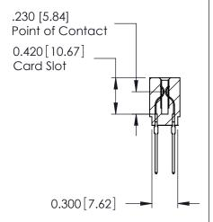
725 Series Ultra-Mate Card Edge Connector - Press Fit Part Number: 725-038-540-201 **EDAC INC** THESE DRAWINGS AND SPECIFICATIONS ARE THE PROPERTY OF EDAC INC.,AND TORONTO, ONTARIO
