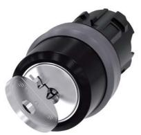
RONIS key-operated switch, 22 mm, round, plastic with metal front ring, special lock, with 2 keys, 2 switch positions O-I, latching, actuating angle 90°, 10:30h/13:30h, key removal O+I, possible special locks: SB31, 421, 455
