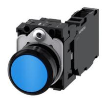
Pushbutton, 22 mm, round, plastic, blue, pushbutton, flat, momentary contact type, with holder 1 NO+1 NC, screw terminal, with laser labeling, symbol number according to, ISO 7000 or IEC 60417
