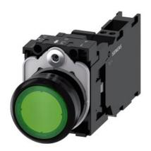
Illuminated pushbutton, 22 mm, round, plastic, green, pushbutton, flat, momentary contact type, with holder, 1 NO+1 NC, LED module with integrated LED 110 V AC, spring-type terminal, with laser labeling, upper case and lower case, always upper case at beginning of line
