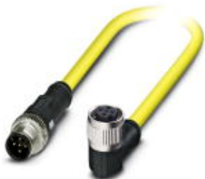
Sensor/actuator cable, 5-position, PVC, yellow, Plug straight M12 SPEEDCON, A-coded, on Socket angled M12 SPEEDCON, A-coded, cable length: 0.5 m
