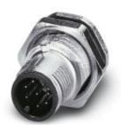
Sensor/actuator flush-type plug, 8-pos., M12-SPEEDCON, shielded, rear/screw mounting with Pg9 thread, with straight solder connection
