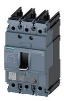
circuit breaker 3VA5 UL frame 125 breaking capacity class S 25kA @ 480V 3-pole, line protection TM230, FTAM, In=100A overload protection Ir=100A fixed short-circuit protection Ii=5...10 x In UL 489 SB (naval), 50° C without connection
