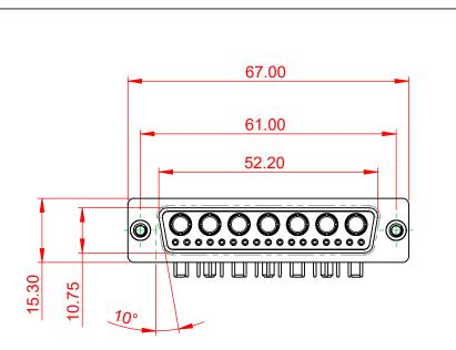
THIS IS A C.A.D. GENERATED DRAWING TOLERANCE UNLESS OTHERWISE SPECIFIED DO NOT MAKE MANUAL REVISIONS TO MASTER. .X ±0.25 .XX ±0.13 .XXX ±0.05
