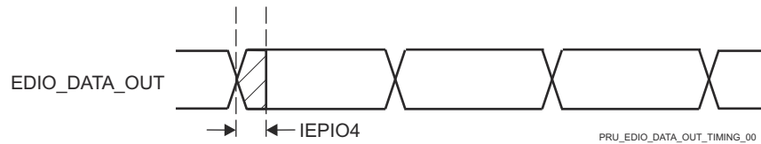
Figure 7-111. PRUSS IEP Digital IOs Timing Requirements
