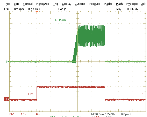
CH1: ILIM, 1V/div, CH4: inductor current, 1A/div, 20ms/div
