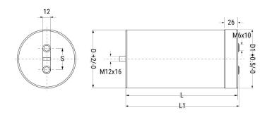
General Information Series C44U-M Dielectric Metallized Polypropylene Style DC Filtering, Energy Storage Features RoHS With Exemptions **REACH** SVHC (Pb - CAS 7439-92-1) SCIP Number cc1c1ec4-db9e-4815-b26b-e8a34ddfb776 Screw Terminals M6 Lead AEC-Q200 No Component 1320 g Weight Thermal Resistance = 3.8 C/W. Weight = 6600 Miscellaneous grams.
