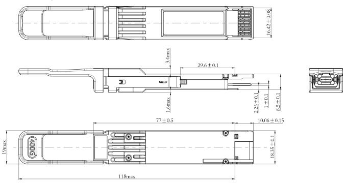
NOTES: 1.TOLERANCE: +/-0.1MM. 2.OTHERS ACCORDING WITH QSFP-DD MSA OR CUSTOMER SPEC. 3.LIGHT PORT ACCORDING WITH FIBER CONNECTOR SPEC.
